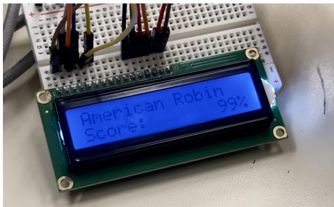
The 60.3 KB classifier running offline on an Arduino Nano 33 BLE Sense.
